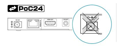
The receiver is powered from the Netvio matrix device over the category cable. A local power supply is not required.
