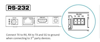
Secure hardwired bi-directional serial control between source and display. Receiver comes complete with 3-Pin screw type connectors for ease of install.
